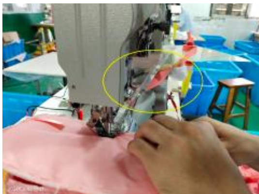
NC-Needle guards were installed but not used correctly for partial high speed sewing machines.jpg
